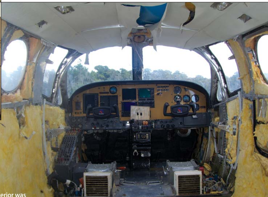
Old interior was completely gutted.
