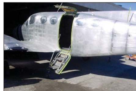
Stripped and ready for painting.
