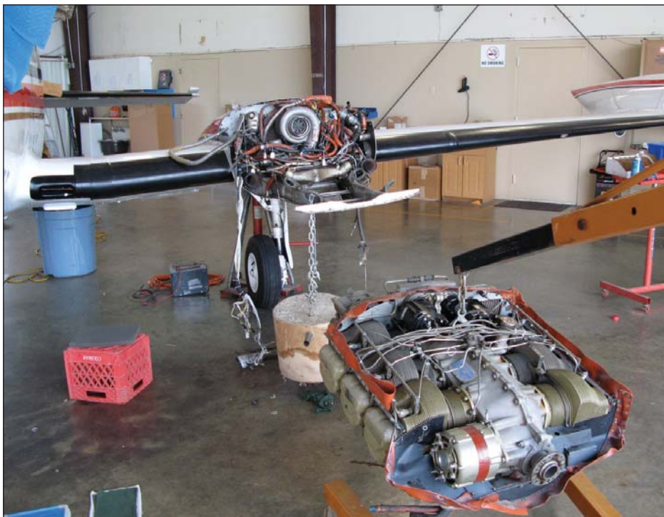
Installing the overhauled engines.
