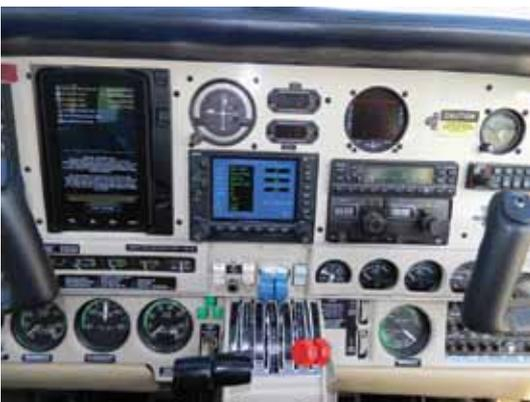
The plane's panel was already fitted with the Garmin 530, so we added an Aspen PFD 1000 PRO, Garmin GTX 330 Transponder, Garmin 340 audio panel, JPI 760, and a Garmin 796 to round things out.
