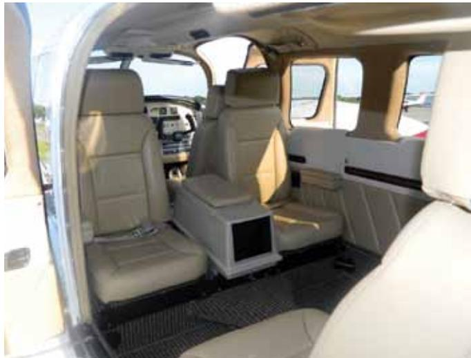
Interior plastic is rather expensive to replace. To save the customer time and money, we wrap existing plastic with fabric. The wrapping not only makes for easier repairs, but also covers up any such repairs for a clean, modern look.
